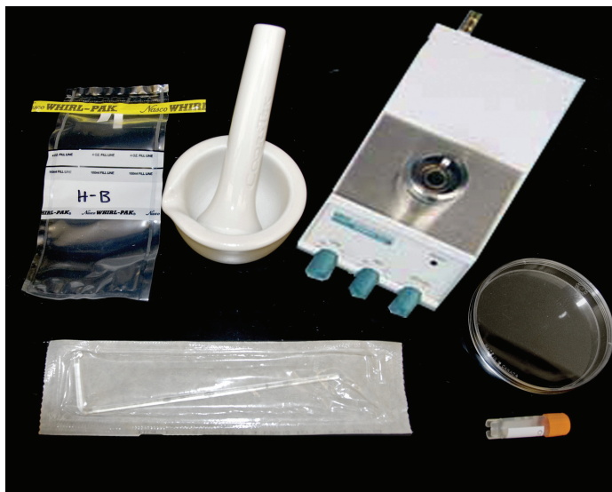
Figure 4.7.2.4 Equipment used in processing tissue samples for microbiology. These include a mortar and pestle for grinding fresh tissue, device to flame sterilize spreading rods, agar plate for culturing bacteria and cryovial for freezing ground tissue sample.
