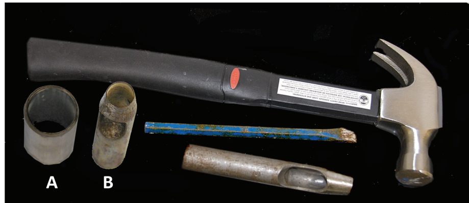
Figure 4.6.6.2 Tools used for bolder corals. Stainless steel coring tube for histology (A) is 2.5 cm, while leather punch (B) biopsy is 1.5 cm.
