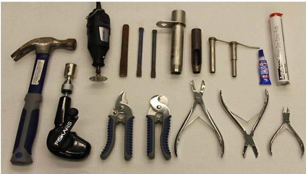
Figure 32. Examples of tools used for fragmenting coral. They include a hammer, a hand drill fitted with a hole saw, a Dremel® rotary tool, various sizes of chisels and corers or leather punches, “coral clippers” similar to pruning shears or bone cutters, and adhesives.
