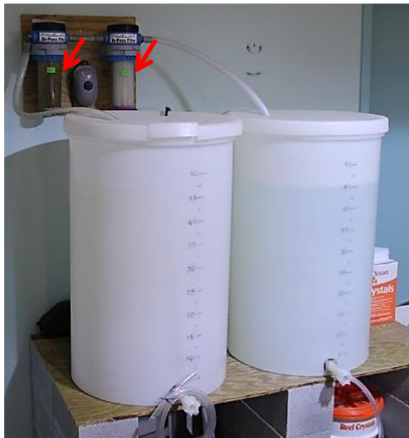
Figure 5. Artificial seawater mixing ( left ) and holding ( right ) tanks. After mixing overnight fresh artificial seawater is pumped through 5 \mu\text{m} and 0.35 \mu\text{m} pleated filters ( arrows ) into the holding tank where it is aerated until use.
