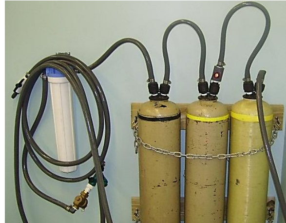
Figure 3. Mixed bed deionizing system for preparing artificial seawater. Tap water passes through a 1 \mu\text{m} pre-filter ( white cylinder ), an activated carbon tank ( black band ), and then through the mixed bed working and polishing deionizer tanks ( yellow bands ). A light indicates when the working tank is spent.
