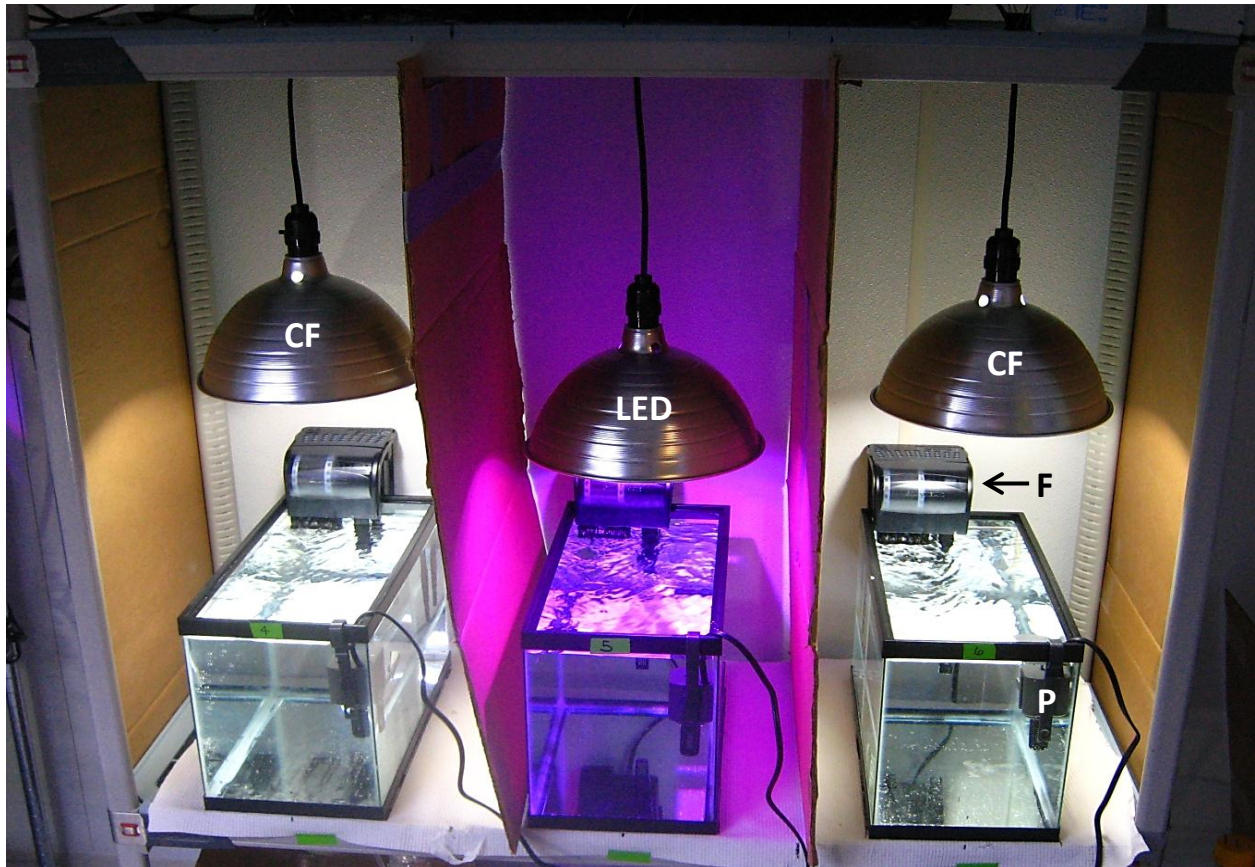
Figure 40. Overview of light experimental setup. Each replicate has its own light source (CF or LED), BIO-Wheel® powerfilter (F) and small powerhead (P) and are separated by cardboard and black plastic sheeting (not shown) to reduce stray light. Only three of the six replicates are shown here.
