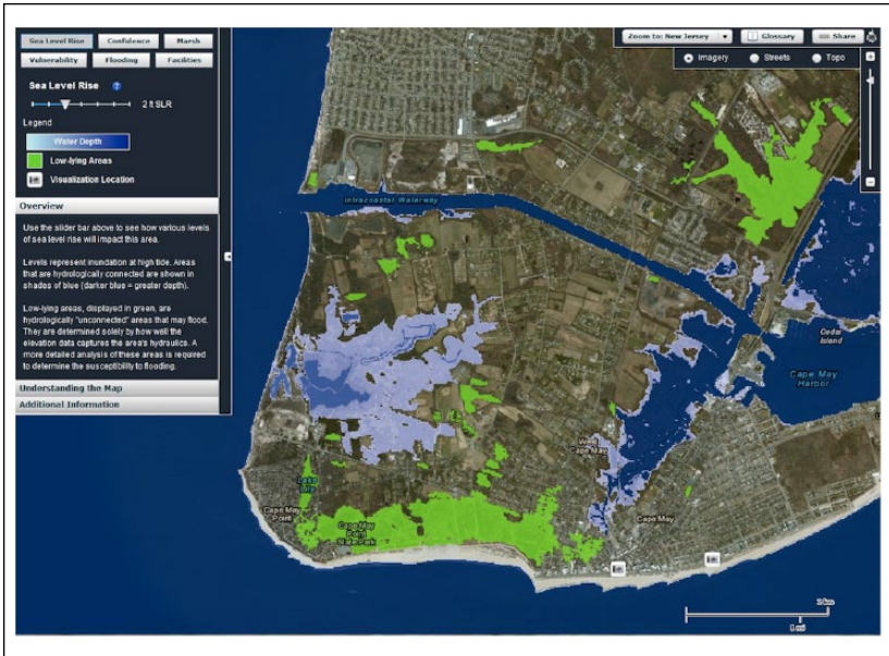
Figure 1. Screenshot from NJ Flood Mapper , showing flooding risks at Cape May, New Jersey, at a 2-foot sea level rise.
