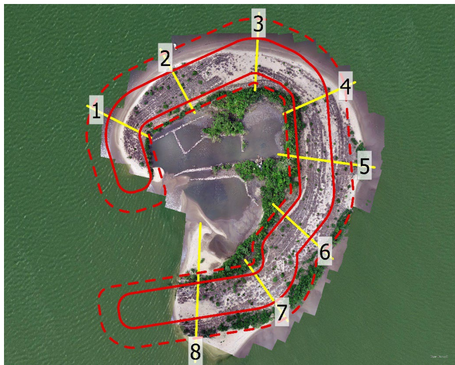
Figure 3. Design plan. Inner, solid polygon indicates the central spine that was designed to 7 ft MLLW. Outer polygon (dashed line) represents full spatial extent of intended project footprint. Perpendicular lines numbered 1-8 represent elevation survey transects occupied in 2023.
