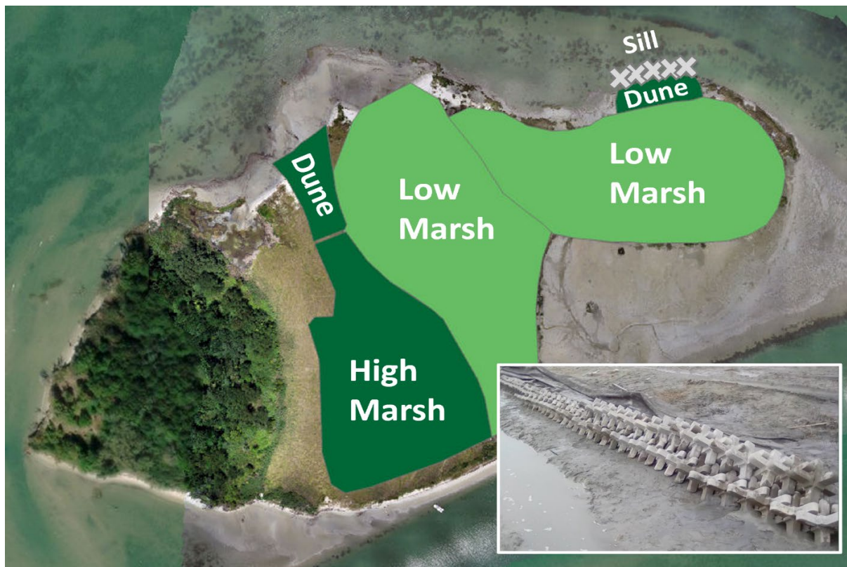
Figure 2. Map of Swan Island indicating relative position of target vegetative communities and Sill. Inset: Sill of stacked A-jacks units.
