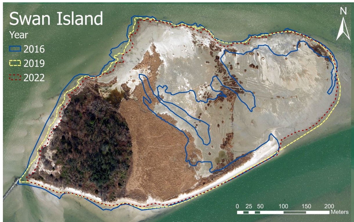
Figure 4. Shoreline position overtime as delineated from aerial imagery. Imagery used to generate these shorelines were 6-inch resolution orthoimages obtained from the MD iMAP system. The background image shown here is from 2022.
