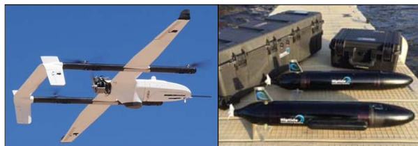
Fig 7. (Left) VTOL sUAS can fly longer and take off and land vertically, making them potentially well suited for ship-based operations.
