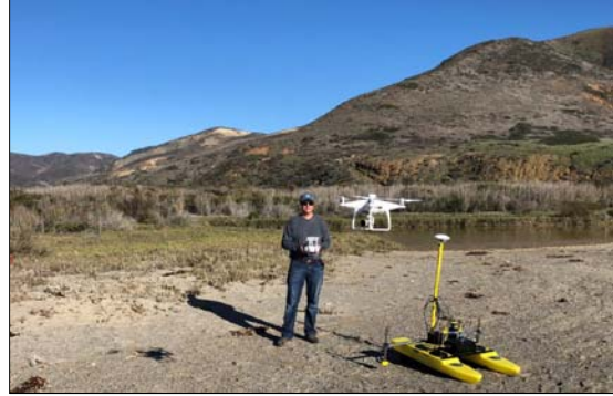
Fig 5. sUAS and ASV deployed in Santa Cruz Island, CA. Data streams from these drones were used to map nearshore depths.
