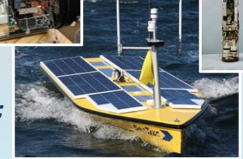
SeaTrac USV + IFCB or 3G ESP: RL 7 prototype w/ IFCB or ESP integrated; operational environment
