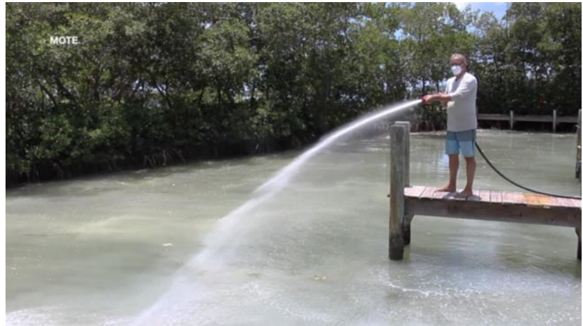
Experimental application of clay flocculation slurry during a small enclosure trial in Sarasota. Note the temporary coloration of the water at the time of application. Credit: Mote Marine Lab.
