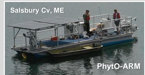
Salsbury Cv, ME Phyto-ARM Towable Barge (solar) (IFCB & 2G spESP co-deployed; profiling CTD)
