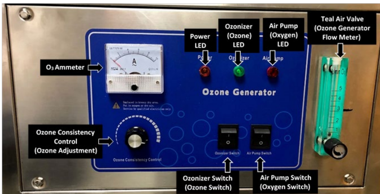
Figure 2. Control panel on the oxygen/ozone generator cabinet of the NBOT 2.5-HP.
