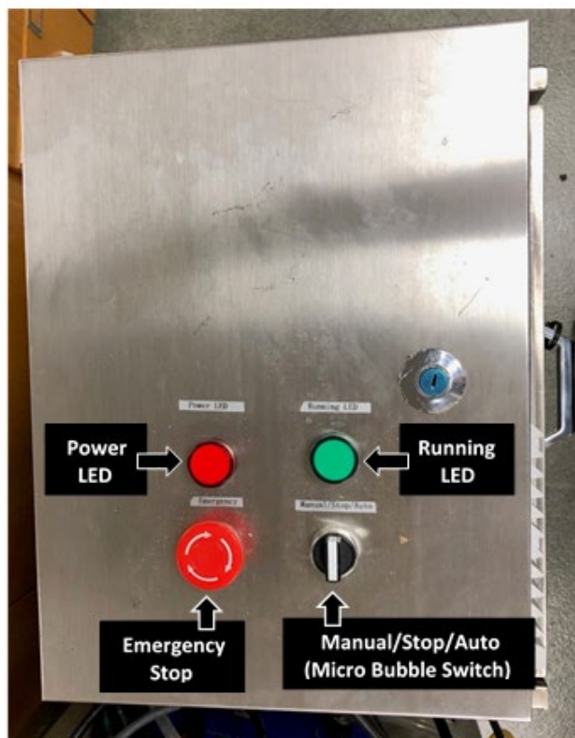
Figure 3. Top view of the pump cabinet of the NBOT 2.5-HP.
