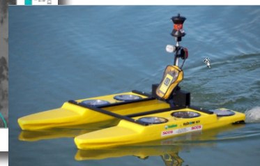
Depth data collected using a single beam sonar mounted on a Hydroner USV in Prisoner's Harbor, Santa Cruz Island, CA; and used to independently validate the depths derived using SfM.
