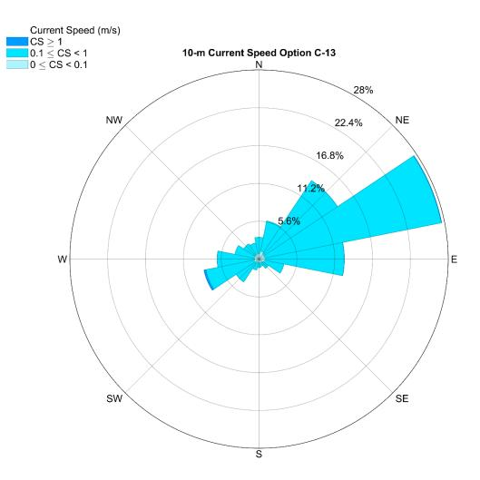
**Figure 3.96.** Ocean current magnitude and direction for option C-13 at 10-m depth. The rose diagram provides percent occurrence for each current speed category. Current flow is in the direction of the compass heading. Data are from the Navy Coastal Ocean Model, Regional American Seas Model (2016 - 2020).
