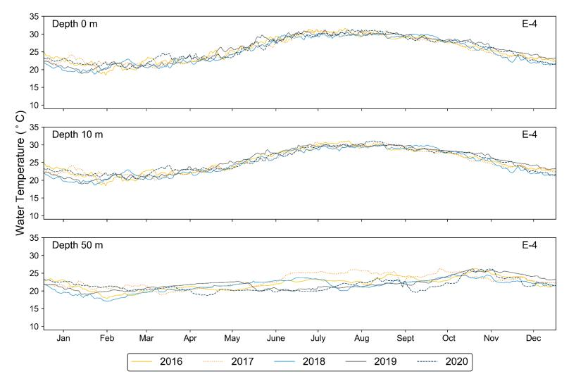
**Figure 3.106.** Option E-4 Navy Coastal Ocean Model regional American seas model mean daily water temperature at the surface, 10-m depth, and 50-m depth (2016 - 2020).
