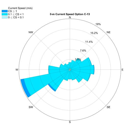
**Figure 3.95.** Ocean current magnitude and direction for option C-13 at the ocean surface. The rose diagram provides percent occurrence for each current speed category. Current flow is in the direction of the compass heading. Data are from the Navy Coastal Ocean Model, Regional American Seas Model (2016 - 2020).
