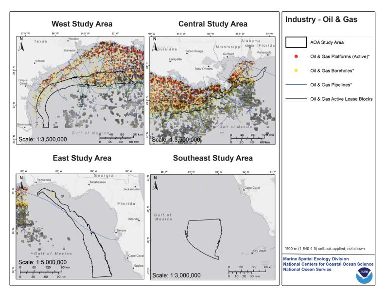
Figure 3.6. Energy infrastructure considerations for the West, Central, East, and Southeast study areas. Considerations include active oil and gas platforms, boreholes and test wells, oil and gas pipelines, and the Bureau of Ocean Energy Management active oil and gas lease blocks.
