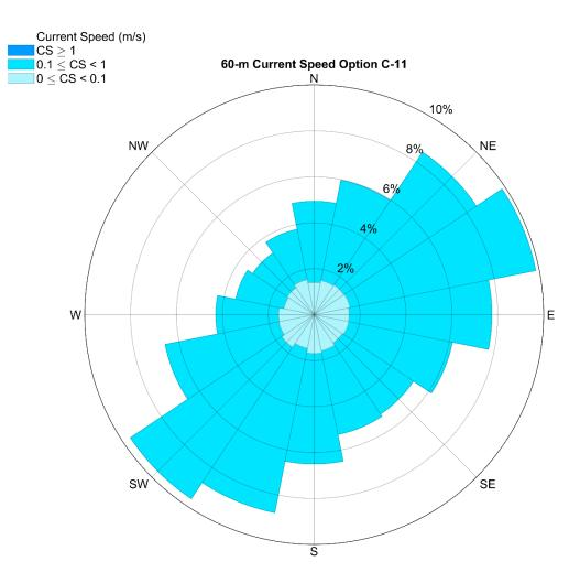
**Figure 3.84.** Ocean current magnitude and direction for option C-11 at 60-m depth. The rose diagram provides percent occurrence for each current speed category. Current flow is in the direction of the compass heading. Data are from the Navy Coastal Ocean Model, Regional American Seas Model (2016 - 2020).
