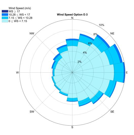
**Figure 3.122.** Wind velocity and direction at 10-m above sea level for option E-3. The rose diagram provides percent occurrence for each wind speed category. Wind direction is displayed as the origin. Wind data are from the North American Regional Reanalysis model (1979 - 2008).
