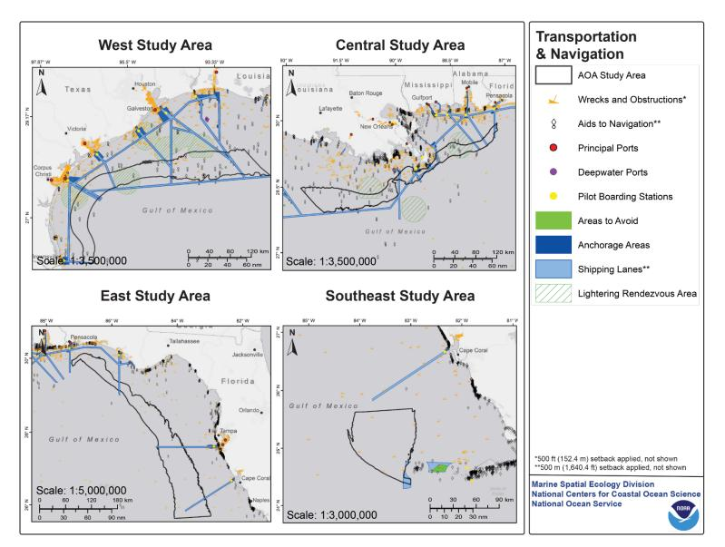
**Figure 3.8.** Transportation and Navigation considerations for the West, Central, East, and Southeast study areas. Considerations include principal ports, shipping infrastructure and routes (e.g., shipping lanes, anchorage areas, pilot boarding stations, deep-water ports, areas to avoid, lightering rendezvous areas, and aids to navigation).
