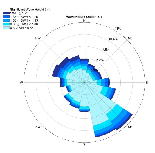
**Figure 3.135.** Significant wave height and direction at 10-m for option E-1. The rose diagram provides percent occurrence for each significant wave height category. Wave direction is displayed as the origin. Wave data are from the MIKE 21 model for the Gulf of Mexico (1979 - 2008).
