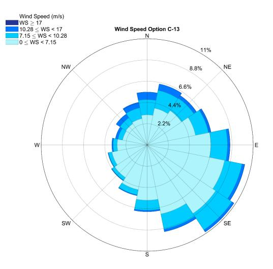
**Figure 3.98.** Wind velocity and direction at 10-m above sea level for option C-13. The rose diagram provides percent occurrence for each wind speed category. Wind direction is displayed as the origin. Wind data are from the North American Regional Reanalysis model (1979 - 2008).
