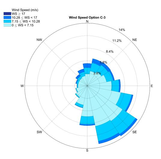
**Figure 3.73.** Wind velocity and direction at 10-m above sea level for option C-3. The rose diagram provides percent occurrence for each wind speed category. Wind direction is displayed as the origin. Wind data are from the North American Regional Reanalysis model (1979 - 2008).
