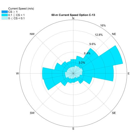
**Figure 3.97.** Ocean current magnitude and direction for option C-13 at 60-m depth. The rose diagram provides percent occurrence for each current speed category. Current flow is in the direction of the compass heading. Data are from the Navy Coastal Ocean Model, Regional American Seas Model (2016 - 2020).
