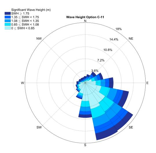
**Figure 3.86.** Significant wave height and direction at 10-m for option C-11. The rose diagram provides percent occurrence for each significant wave height category. Wave direction is displayed as the origin. Wave data are from the MIKE 21 model for the Gulf of Mexico (1979 - 2008).
