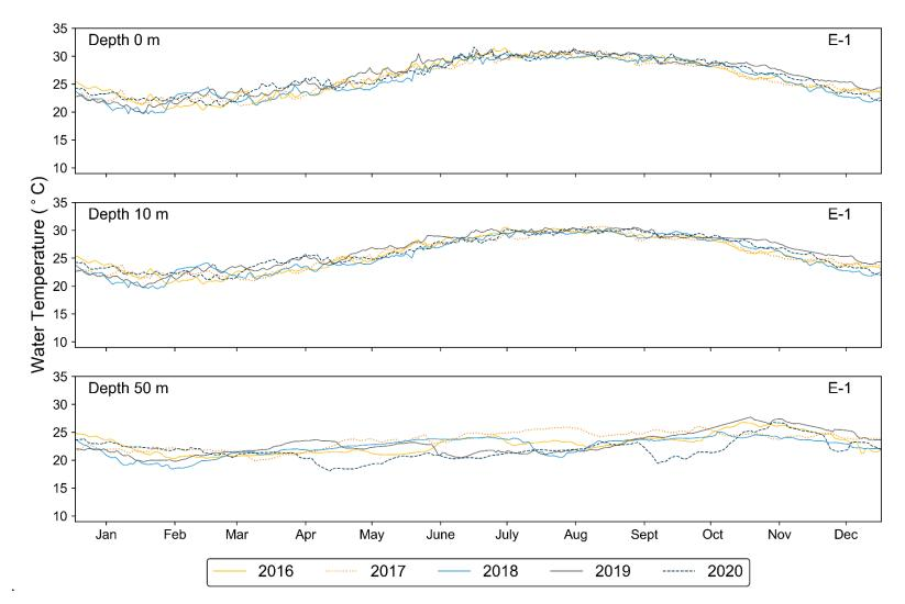
**Figure 3.130.** Option E-1 Navy Coastal Ocean Model regional American seas model mean daily water temperature at the surface, 10-m depth, and 50-m depth (2016 - 2020).
