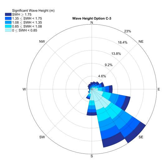
**Figure 3.74.** Significant wave height and direction at 10-m for option C-3. The rose diagram provides percent occurrence for each significant wave height category. Wave direction is displayed as the origin. Wave data are from the MIKE 21 model for the Gulf of Mexico (1979 - 2008).
