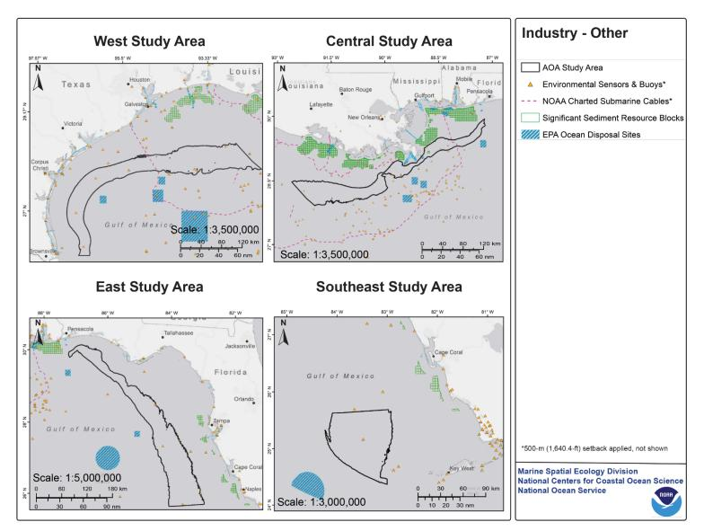
**Figure 3.7.** Ocean infrastructure considerations for the West, Central, East, and Southeast study areas. Considerations include USEPA ocean disposal sites, submarine cables, environmental sensors and buoys, and the Bureau of Ocean Energy Management significant sediment resource blocks.
