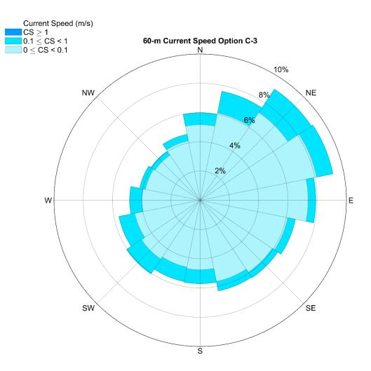
**Figure 3.72.** Ocean current magnitude and direction for option C-3 at 60-m depth. The rose diagram provides percent occurrence for each current speed category. Current flow is in the direction of the compass heading. Data are from the Navy Coastal Ocean Model, Regional American Seas Model (2016 - 2020).
