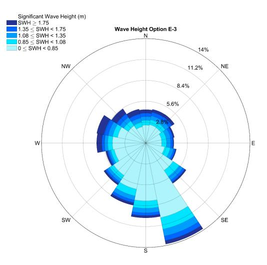
**Figure 3.123.** Significant wave height and direction at 10-m for option E-3. The rose diagram provides percent occurrence for each significant wave height category. Wave direction is displayed as the origin. Wave data are from the MIKE 21 model for the Gulf of Mexico (1979 - 2008).
