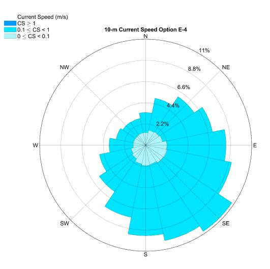
**Figure 3.108.** Ocean current magnitude and direction for option E-4 at 10-m depth. The rose diagram provides percent occurrence for each current speed category. Current flow is in the direction of the compass heading. Data are from the Navy Coastal Ocean Model, Regional American Seas Model (2016 - 2020).
