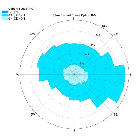
**Figure 3.71.** Ocean current magnitude and direction for option C-3 at 10-m depth. The rose diagram provides percent occurrence for each current speed category. Current flow is in the direction of the compass heading. Data are from the Navy Coastal Ocean Model, Regional American Seas Model (2016 - 2020).
