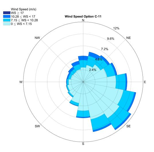
**Figure 3.85.** Wind velocity and direction at 10-m above sea level for option C-11. The rose diagram provides percent occurrence for each wind speed category. Wind direction is displayed as the origin. Wind data are from the North American Regional Reanalysis model (1979 - 2008).
