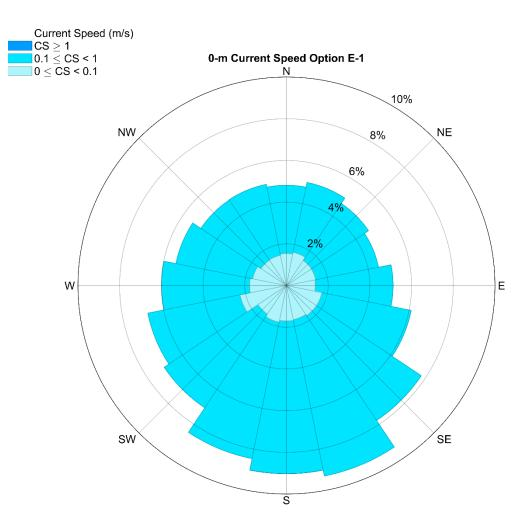
**Figure 3.131.** Ocean current magnitude and direction for option E-1 at the ocean surface. The rose diagram provides percent occurrence for each current speed category. Current flow is in the direction of the compass heading. Data are from the Navy Coastal Ocean Model, Regional American Seas Model (2016 - 2020).
