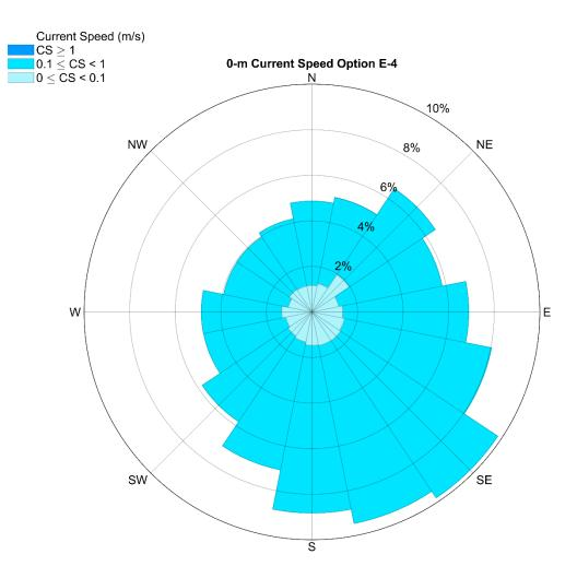
**Figure 3.107.** Ocean current magnitude and direction for option E-4 at the ocean surface. The rose diagram provides percent occurrence for each current speed category. Current flow is in the direction of the compass heading. Data are from the Navy Coastal Ocean Model, Regional American Seas Model (2016 - 2020).
