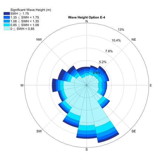
**Figure 3.111.** Significant wave height and direction at 10-m for option E-4. The rose diagram provides percent occurrence for each significant wave height category. Wave direction is displayed as the origin. Wave data are from the MIKE 21 model for the Gulf of Mexico (1979 - 2008).
