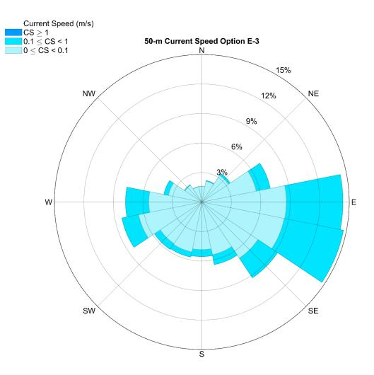
**Figure 3.121.** Ocean current magnitude and direction for option E-3 at 50-m depth. The rose diagram provides percent occurrence for each current speed category. Current flow is in the direction of the compass heading. Data are from the Navy Coastal Ocean Model, Regional American Seas Model (2016 - 2020).
