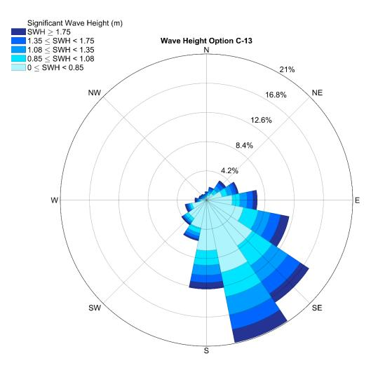
**Figure 3.99.** Significant wave height and direction at 10-m for option C-13. The rose diagram provides percent occurrence for each significant wave height category. Wave direction is displayed as the origin. Wave data are from the MIKE 21 model for the Gulf of Mexico (1979 - 2008).
