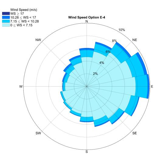
**Figure 3.110.** Wind velocity and direction at 10-m above sea level for option E-4. The rose diagram provides percent occurrence for each wind speed category. Wind direction is displayed as the origin. Wind data are from the North American Regional Reanalysis model (1979 - 2008).
