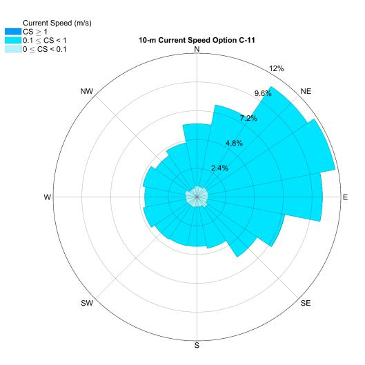
**Figure 3.83.** Ocean current magnitude and direction for option C-11 at 10-m depth. The rose diagram provides percent occurrence for each current speed category. Current flow is in the direction of the compass heading. Data are from the Navy Coastal Ocean Model, Regional American Seas Model (2016 - 2020).
