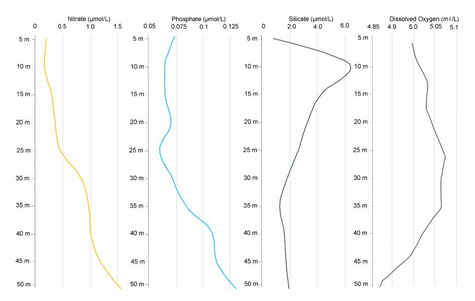
**Figure 3.124**. Option E-3 concentration of dissolved nitrate, phosphate, silicate and oxygen at different depth levels derived from the Ecological Marine Units (Sayre et al. 2017).
