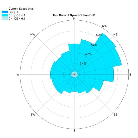
**Figure 3.82.** Ocean current magnitude and direction for option C-11 at the ocean surface. The rose diagram provides percent occurrence for each current speed category. Current flow is in the direction of the compass heading. Data are from the Navy Coastal Ocean Model, Regional American Seas Model (2016 - 2020).
