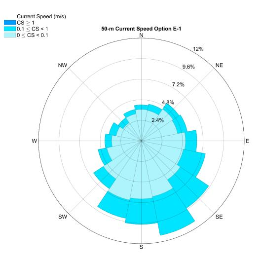
**Figure 3.133.** Ocean current magnitude and direction for option E-1 at 50-m depth. The rose diagram provides percent occurrence for each current speed category. Current flow is in the direction of the compass heading. Data are from the Navy Coastal Ocean Model, Regional American Seas Model (2016 - 2020).
