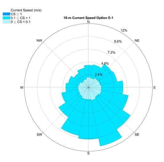
**Figure 3.132.** Ocean current magnitude and direction for option E-1 at 10-m depth. The rose diagram provides percent occurrence for each current speed category. Current flow is in the direction of the compass heading. Data are from the Navy Coastal Ocean Model, Regional American Seas Model (2016 - 2020).
