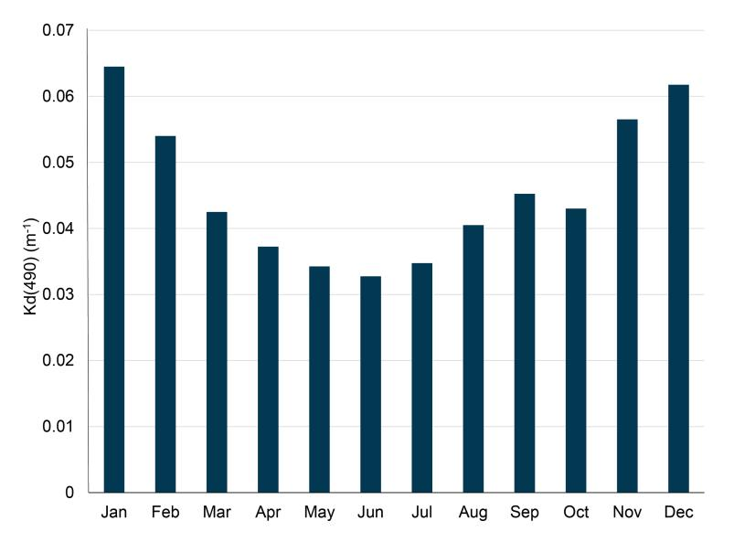
**Figure 3.138.** Option E-1 monthly climatological mean (2010 - 2017) for Kd(490) within the top meter of water produced by Visible Infrared Imaging Radiometer Suite 750-m data.
