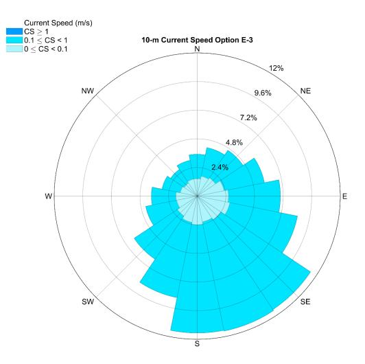
**Figure 3.120.** Ocean current magnitude and direction for option E-3 at 10-m depth. The rose diagram provides percent occurrence for each current speed category. Current flow is in the direction of the compass heading. Data are from the Navy Coastal Ocean Model, Regional American Seas Model (2016 - 2020).
