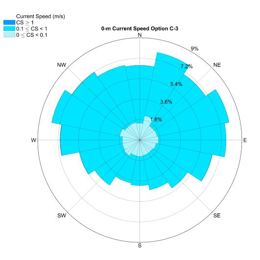
**Figure 3.70.** Ocean current magnitude and direction for option C-3 at the ocean surface. The rose diagram provides percent occurrence for each current speed category. Current flow is in the direction of the compass heading. Data are from the Navy Coastal Ocean Model, Regional American Seas Model (2016 - 2020).
