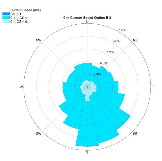
**Figure 3.119.** Ocean current magnitude and direction for option E-3 at the ocean surface. The rose diagram provides percent occurrence for each current speed category. Current flow is in the direction of the compass heading. Data are from the Navy Coastal Ocean Model, Regional American Seas Model (2016 - 2020).
