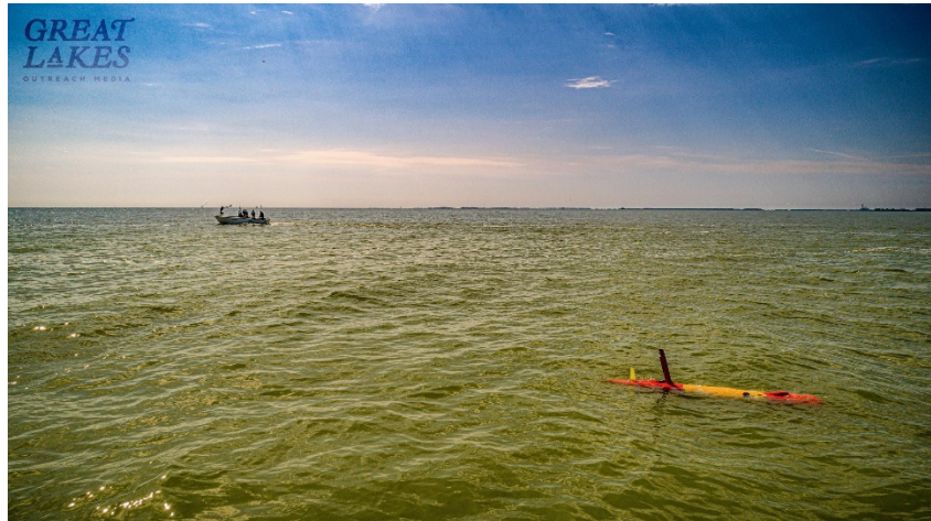
Figure 5. Scientists from NOAA and Monterey Bay Aquarium Research Institute (MBARI) aboard a NOAA research vessel deploying a long-range autonomous underwater vehicle (LRAUV) in Lake Erie's HAB. This LRAUV's mission is to map algae concentrations throughout the bloom and tell the 3rd generation environmental sample processor (3GESP) where to measure microcystin toxin levels. Image credit: David J Ruck, Great Lakes. Outreach Media.
