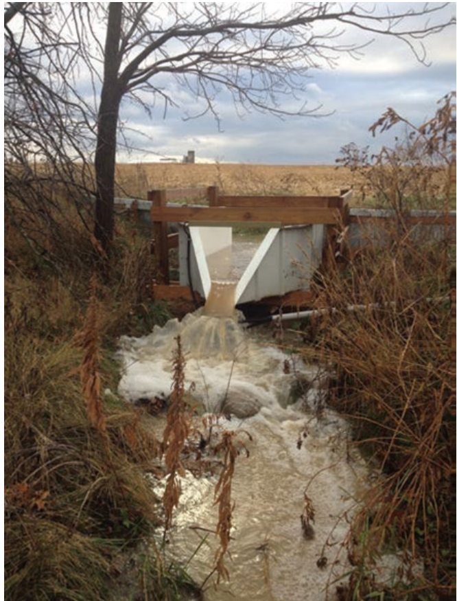
Figure 12. Example of a USDA edge-of-field water quality monitoring station in Ohio.
