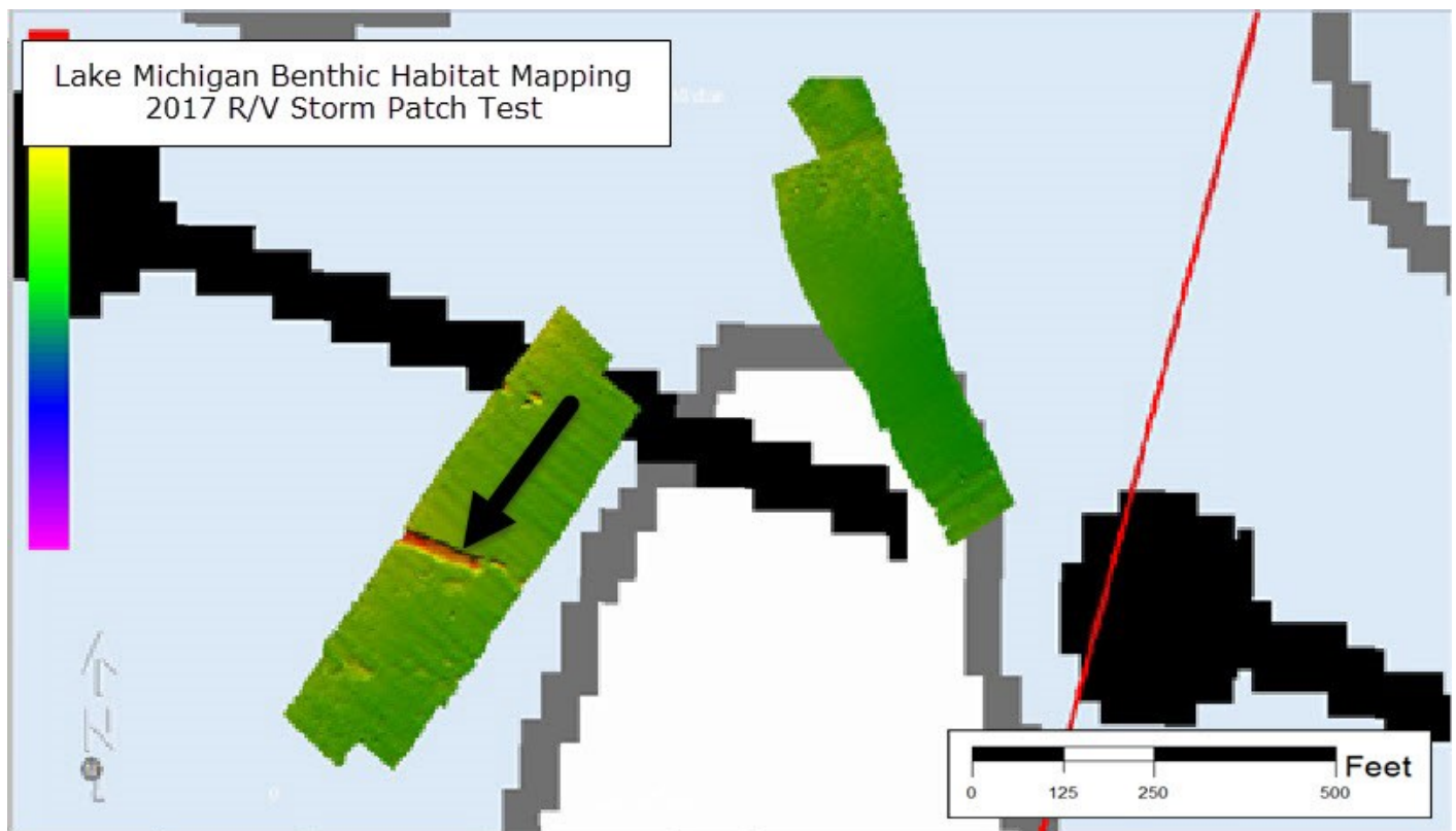
Figure 3. Patch test conducted over the Manitowoc Waterworks plant pipeline. Notice the structure was detected nearly 200 feet to the south of the charted position of the pipeline.
