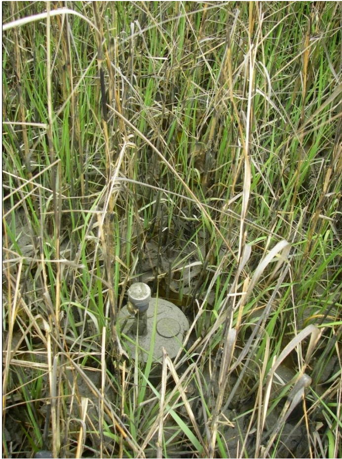
Figure 10. Photo of a Class B Benchmark where the SET receiver (see Figure 6) is mounted to support Surface Elevation Table readings. Diameter of PVC collar is 6 inches. PVC cap covers the receiver, and a brass marker is placed in the concrete identifying the benchmark.
