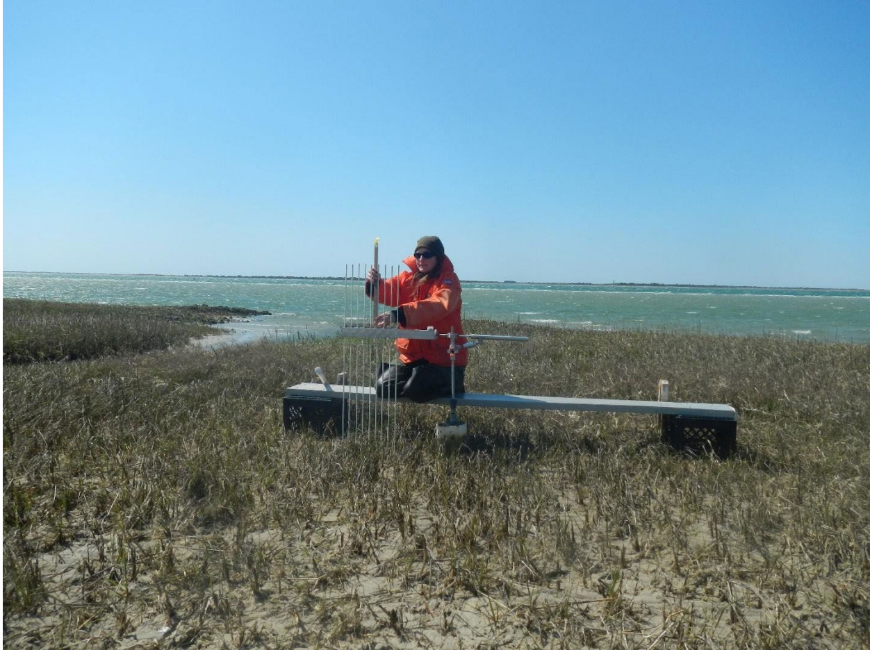
Figure 6. Photo of a surface elevation table (SET) instrument mounted on a benchmark (see Figure 10). A temporary boardwalk is shown being used by the scientist to access a benchmark without walking on marsh surface. The distance to marsh is read with the fiberglass rods. Only the benchmark (small PVC-capped object in center of photo) remains in the marsh.
