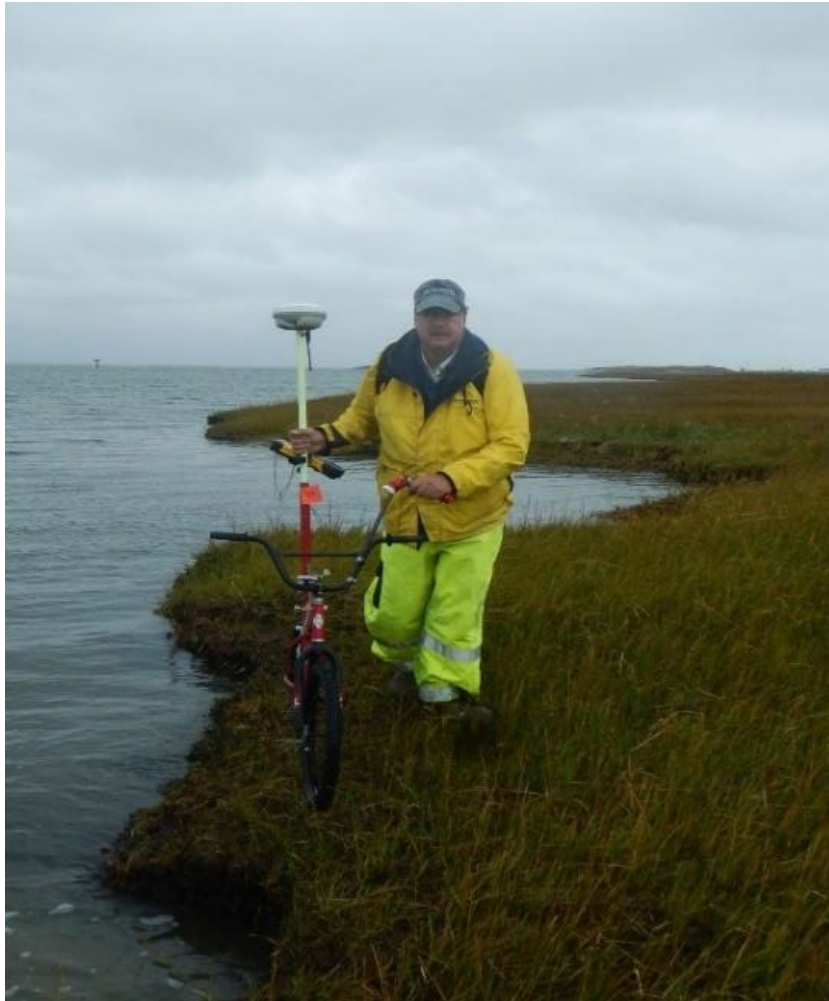
Figure 2. RTK marsh survey with bike mounted rover. Base receiver is occupying a surveyed benchmark position.
