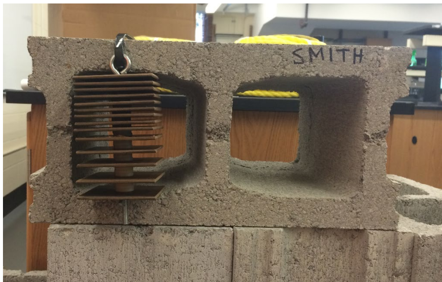
Figure 7. Image of Hester-Dendy samplers placed within a cinder block and ready for deployment. A marker buoy may or may not be attached.
