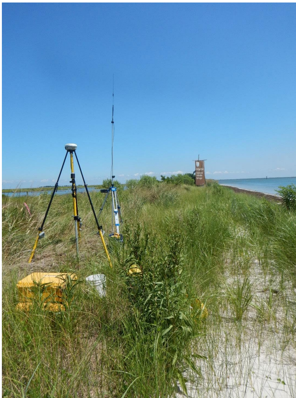
Figure 11. Photo of RTK (Real-time Kinematic) GPS gear set up on an elevation benchmark to accommodate elevation surveys of the site.
